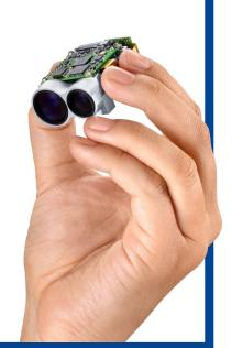
The LRF3013 is very compact and extremely powerful and measures conveniently up to more than 5 km. In addition it is highly shock-resistant and withstands the harshest weapon shocks up to 1600 g.
